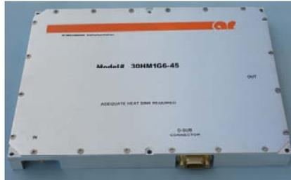
The Model 30HM1G6-45 is a compact, wide-band, hybrid power amplifier module that covers 0.7-6GHz. When used with a sweep generator, the Model 30HM1G6-45 provides a minimum of 30W of RF power instantaneously from 0.7-6 GHz with  $RF_{IN} = 0dBm$ .
